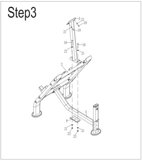
1. Align the support pipe weldment (5), arc plate 1 (8) and rear connecting frame (4) with the hole according to the figure M10\*65 pan head hexagon bolt (18),  $\Phi$ 10 flat gasket (21), M10 locknut (23) to lock itStay, donot lock.
