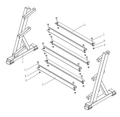
Put component 1 and 2 according to the figure, and use hex bolts M12\*60 (7), flat cushion D12 (8) and anti-loose nut M12 (9) to connect mounting plate (3) with (1) (2) as shown in the figure.
